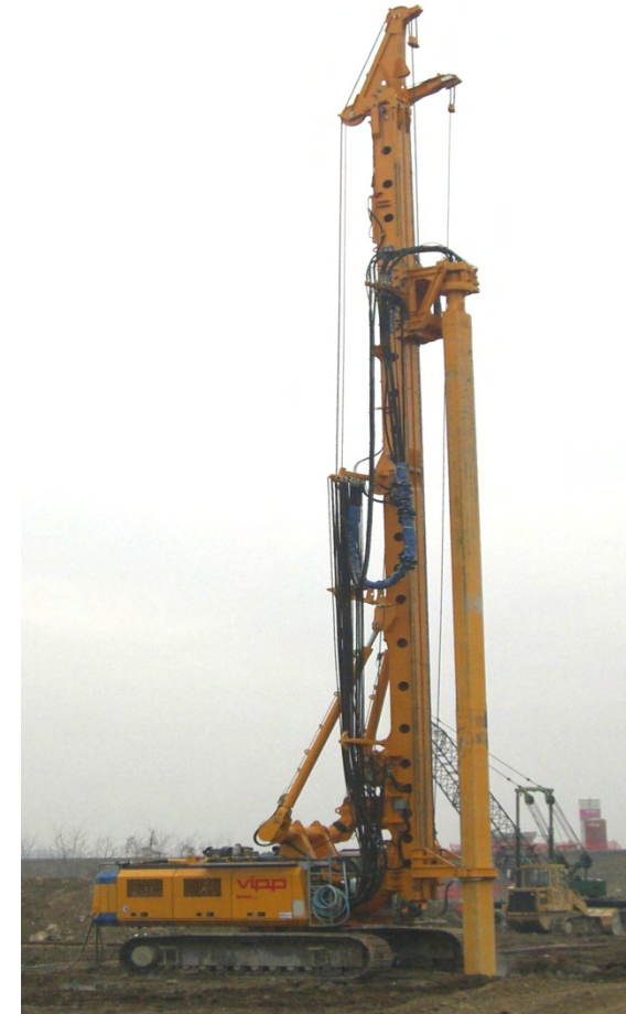
drilling rig BG 28 T = 23 m
