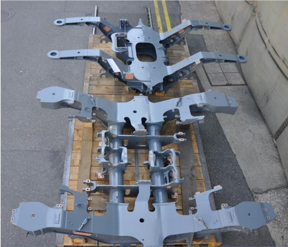
-40% SF900 lightweight frame High strength steel
