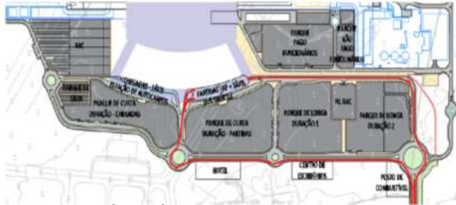
Circulation flow of private vehicles using the very short stay passenger drop off zone in the departures area (“Kiss & Fly”)
