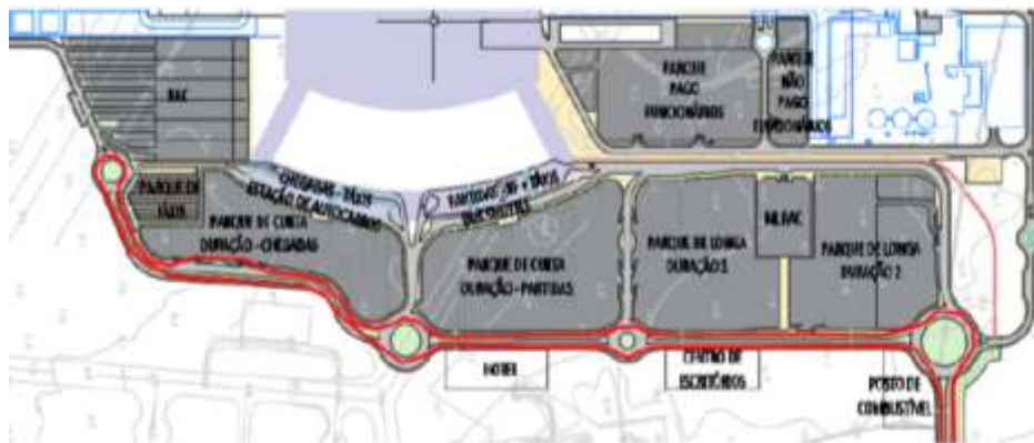
Circulation flow of private vehicles inbound and outbound to/from the short stay car park in the arrivals area
